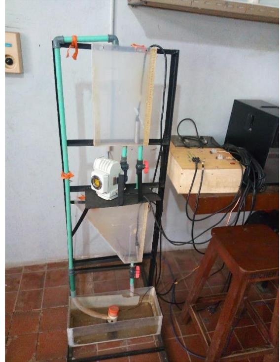
Plate 1: Experimental Setup of cascaded two tank system
