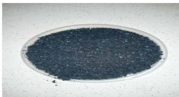
Plate 1: Synthesized AC produced from PVC under optimized conditions from PVC
