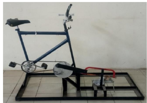
Figure 5: Fabricated pedal powered hacksaw
