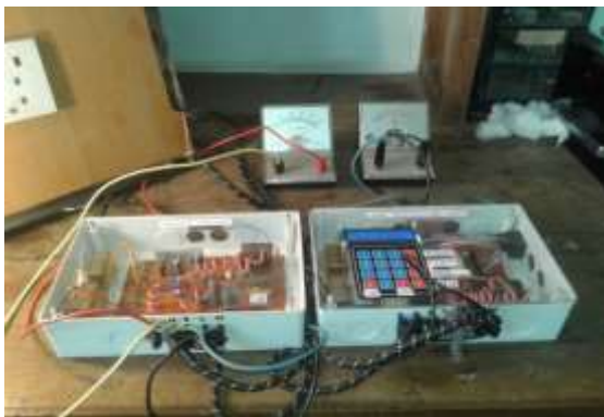
Figure 8 Smart meter being tested in the laboratory
