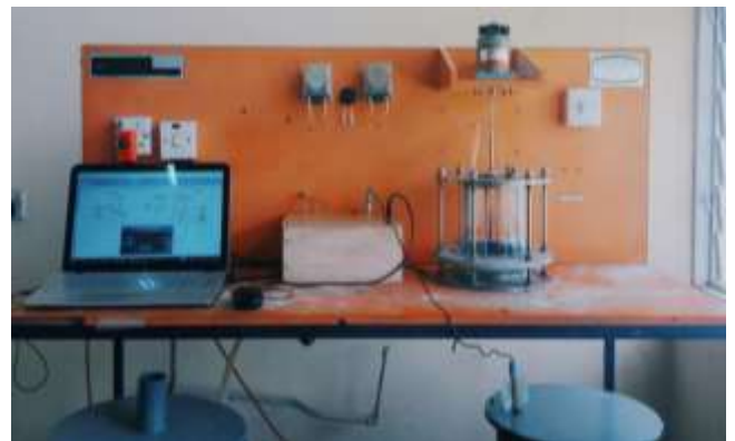
Figure 3: Laboratory scale pH neutralization system
