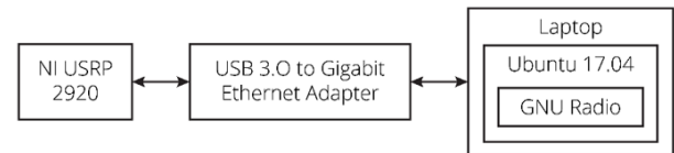
Figure 2. System block diagram
