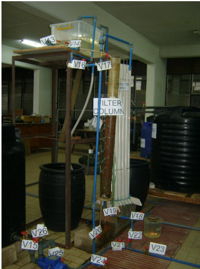
Plate 3: Laboratory set-up for the filtration experiment
