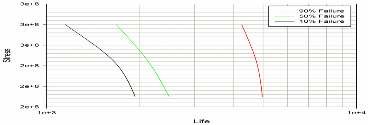
Figure 8: Probability-stress-life plot for annealed specimens
