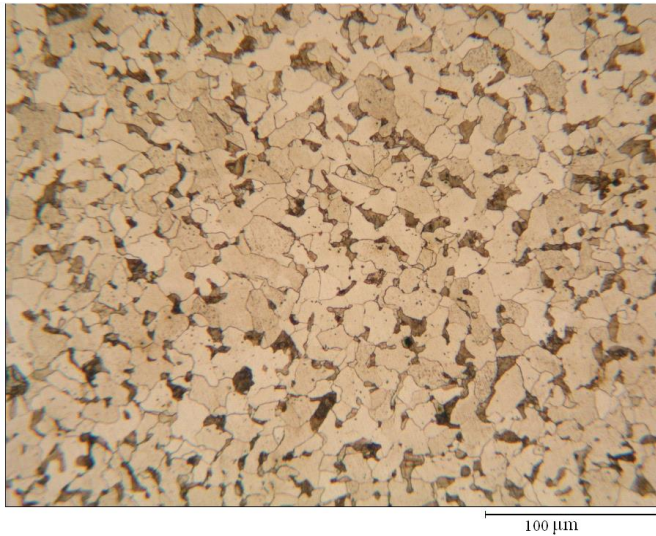
Figure 1: Optical microscope image of API 5L X65 carbon steel after being polished and etched in 2% nital solution for 10 seconds (dark background = pearlite and lighter background = ferrite)
